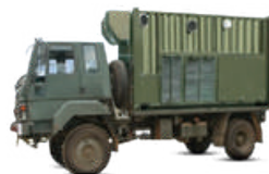
Military Containerized Shelter Truck
